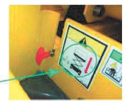
N.B.-:-Pulling on to the T-Handle, immediately activates the emergency lowering of the platform.
