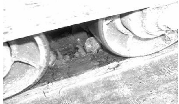
Results of Running in Heavy Rock Condition
