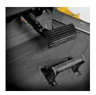
Choose the decelerator function that's right for the job. Slow both ground speed and engine rpm, or ground speed only to help maintain traction without affecting engine power and hydraulic response. Fully depressing the pedal applies the brakes.
