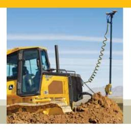
With optional Integrated Grade Control (IGC), your 650J Dozer arrives from the factory "plug and play" ready. Its open architecture design lets you employ the electronic grade-control system that's right for you.
