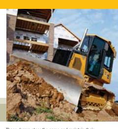
These dozers steer the same and maintain their preset speed whether they're on level ground or a 2-to-1 slope. For total control regardless of the terrain.
