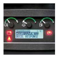
Exclusive TMC lets you customize decelerator mode and response, forward/reverse ground-speed ranges, steering modulation, FNR shift rate, and forward/reverse speed ratios, for unsurpassed control.
