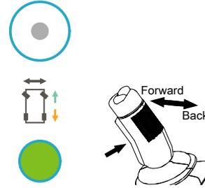
1. Move the lift-drive toggle switch backward to select drive. The "drive enabled" light should illuminate.
