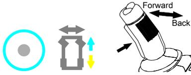
1. Press the drive/steer function button. The button should illuminate.
