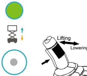
1. Move the lift-drive toggle switch forward to select lift. The "lift enabled" light should illuminate.
