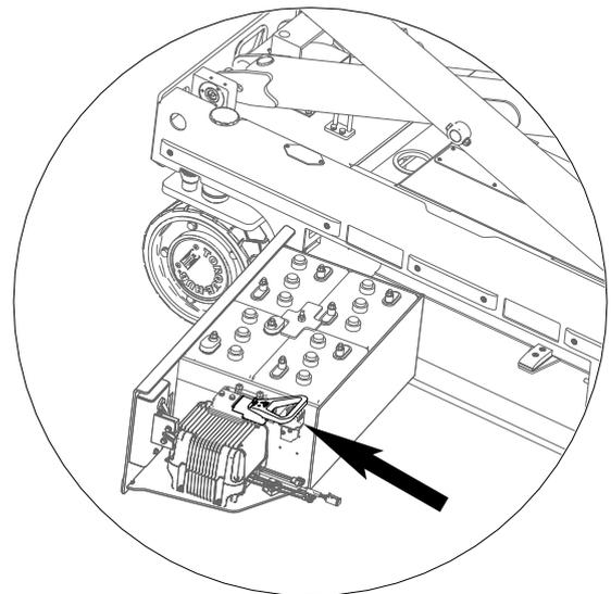
**Figure 7-1 Power disconnect plug assembly**
